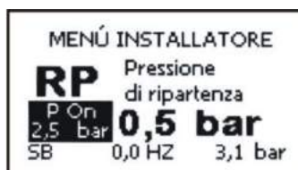
Figure 14: Setting the restart pressure
