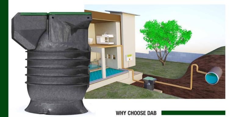
Automatic collection and lifting station suitable for lifting clear and rain water, as well as water loaded with civil and industrial waste. It consists of a cylindrical polyethylene monobloc, and an appropriately shaped bottom for the housing of the pump and for avoiding water stagnation. The upper rectangular opening has polyethylene covers with locking system and smell prevention seals.
