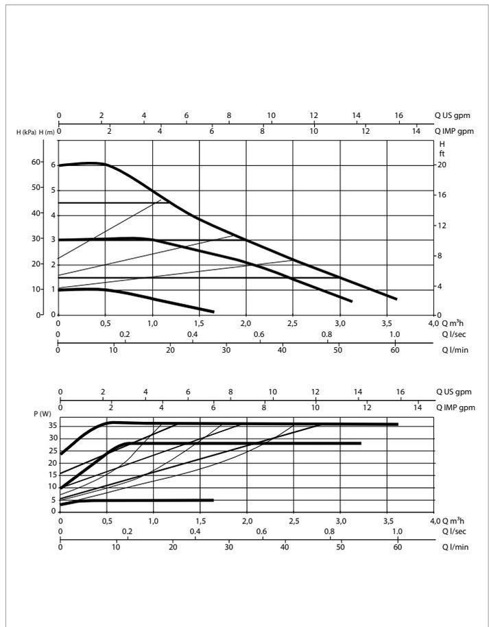
The performance curves are based on kinematic viscosity values = 1 mm<sup>2</sup>/s and density equal to 1000 kg/m<sup>3</sup>. Curve tolerance according to ISO 9906.
