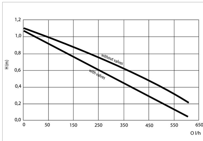
The performance curves are based on kinematic viscosity values = 1 mm<sup>2</sup>/s and density equal to 1000 kg/m<sup>3</sup>. Curve tolerance according to ISO 9906.
