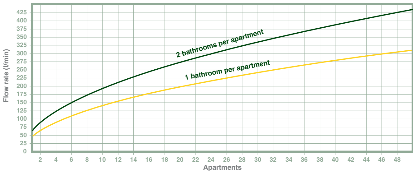
TOILET FLUSHING TAPS
