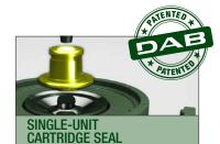
A single-unit cartridge seal is a great advantage for maintenance of the pump as allows the removal and insertion of the seals in less time, having a total guarante to carry out properly. It's an **exclusive patent DAB**: a double mechanical seal Sic-Sic with opposite faces, independent from the rotation direction of shaft, with Viton elastomers and leap seal.
