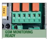
Possible connection to a GSM card for SMS control of the status of the pumps and the panel.
