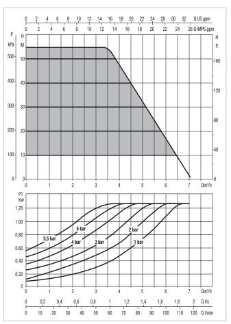
The performance curves are based on kinematic viscosity values =  $1 \text{ mm}^2/\text{s}$  and density equivalent to 1000 kg/m<sup>3</sup>. Curve tolerance according to ISO 9906.
