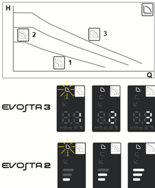
In this regulating mode the circulator works on characteristic curves at a constant speed.
