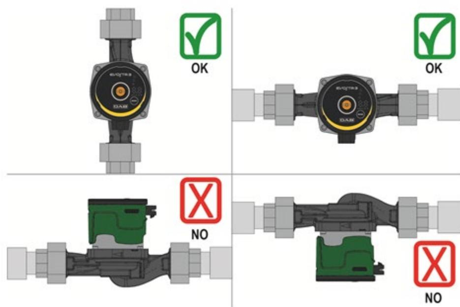
Fig. 3: Monteringsposition
