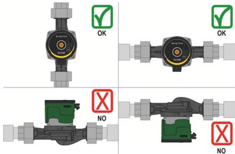
Figure 3: Assembly position
