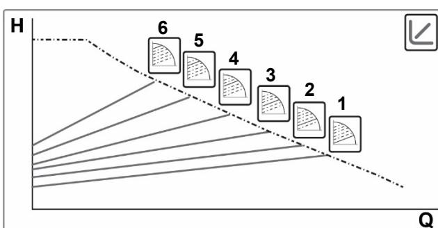
Holding down the Mode key for 20" gives access to the Advanced Menu with the possibility of selecting from 6 curves with proportional differential pressure
