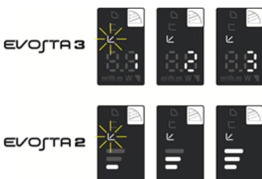
In this regulating mode the differential pressure is reduced or increased as the demand for water decreases or increases.
