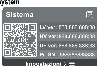
The screen shows the parameters identifying the inverter and its firmware versions on the right, and a QR-code containing more product identification data on the left.
