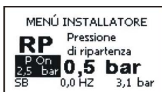
Figure 10: Setting the restart pressure
