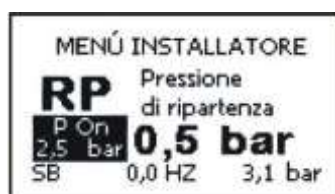
Figure 16: Setting the restart pressure
