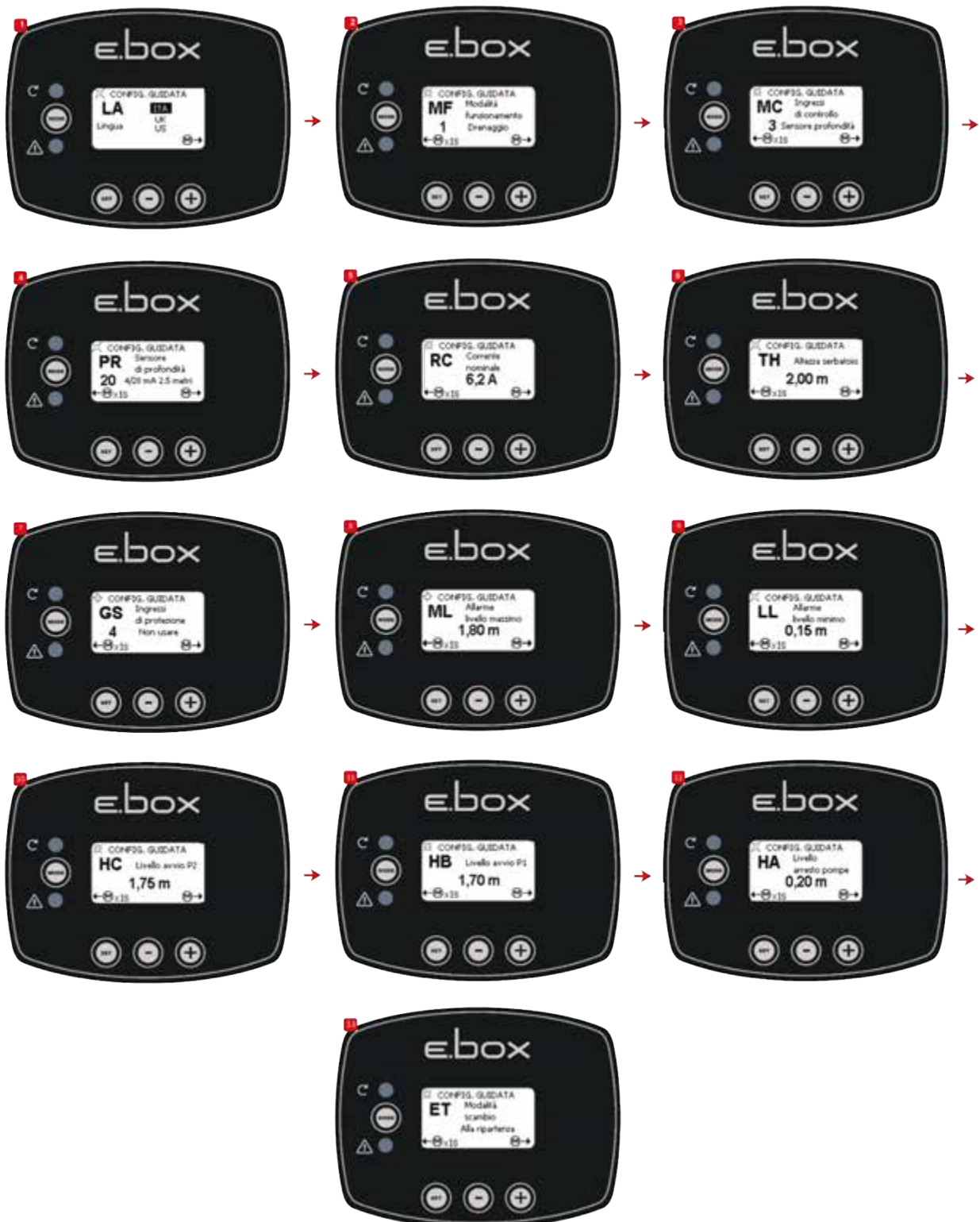
Figure 38: Configuration with only a depth sensor
