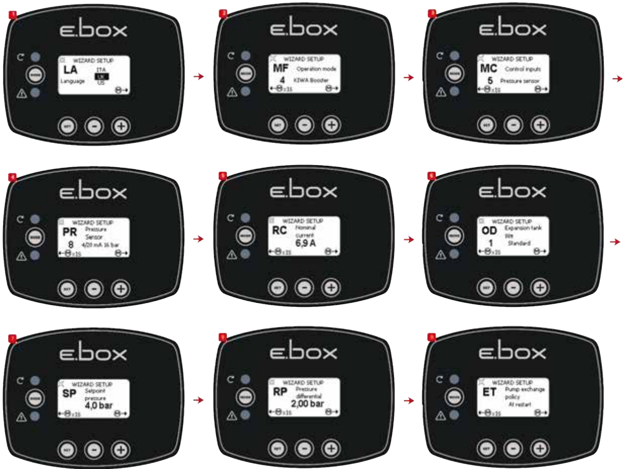
Figure 48: KIWA pressure boosting with pressure sensor
