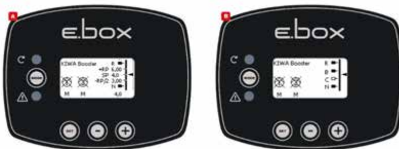
Figure 50: System status in KIWA mode
