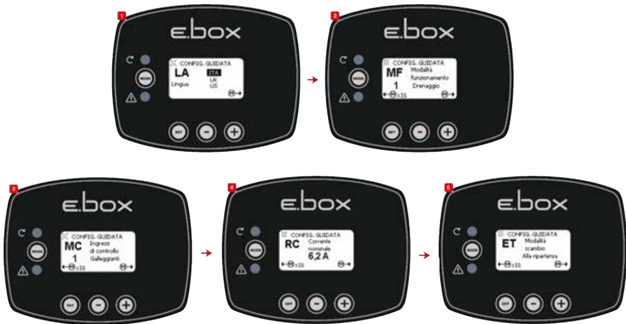
Figure 36: Configuration of Drainage floats or level probes
